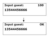
If the countdown reaches 0 before the next guest calls turn the power off and then back on to re-enter programming mode. After you have finished programming turn off the unit and remove the 12V source from terminal 15 and ground. Then turn it back on for normal operation.
