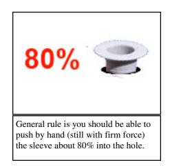
Next stand your fence upright in the holes with sleeves in them. When you are first installing the fence expect there to be tension to reach from base of pole to base of pole. <u>Tension at the top of the poles however is not achieved until after the sections of fence are fully attached to one another by hook and eyes.</u>
