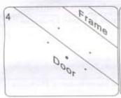
Drill two holes in the frame and three holes in the door as indicated on the template.
