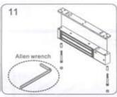
Use the Allen wrench to screw the Fixing screws and Brass Sleeves through the bottom of the electromagnet into the mounting plate.
