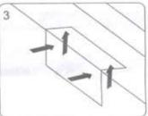
Place the template against the door and frame. Drill two holes in the frame and three holes in door as indicated on the template.
