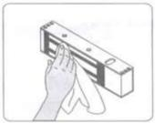
Apply a light coat of a silicon lubricant to prevent rust. Wipe away the excess.
