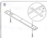
Screw the two self-tapping screws in the slotted holes of the mounting plate and adjust the position of the mounting plate so that it and the armature plate from a 90-degree angle.
