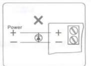
Do not install a diode in parallel with any magnetic lock. A diode will cause a delay when releasing the door and residual magnet to occur.
