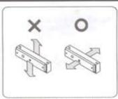
During the installation procedure, it is important to make sure that the working direction of the armature plate has to be facing toward the contact surface of the electromagnetic lock intend to have the maximum holding force.
