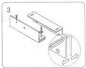
Assemble the Z bracket, and make sure that the Z bracket is adjustable.
