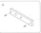
Insert the guide pins into the armature plate. The guide pins will prevent the armature plate to pivot around.
