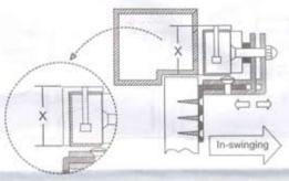
The "X" value in the table below for each bracket to mount on the door frame, shows the minimum requirement width of the door frame for different electromagnetic lock model.
