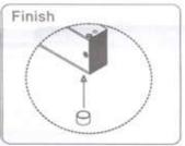
Insert the anti-tamper caps into the mounting screw access holes. This should be the last step, as once the tamper caps are in place, they will be difficult to remove.
