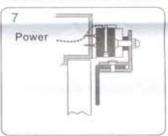
Turn on the power of EM-Lock, and let the armature plate bonds to the EM-lock. Adjust the position between the Z bracket and the door frame.
